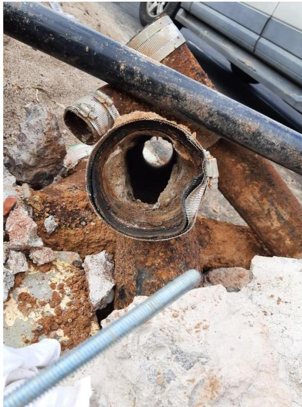
*A pipe with significant FOG accumulation*
